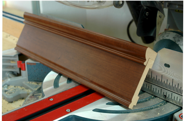
This cherry-look wrap is applied to wide, two-part trim. The MDF substrate is visible on the end. Photo credit: Steve Maxwell
