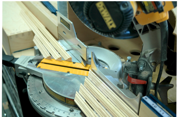
A mitre saw is the ideal tool for making trim and moulding easier to install. Here one end of 7 pieces of trim have been cut to an angle in preparation for marking and final cutting of the second ends. Photo credit: Steve Maxwell
